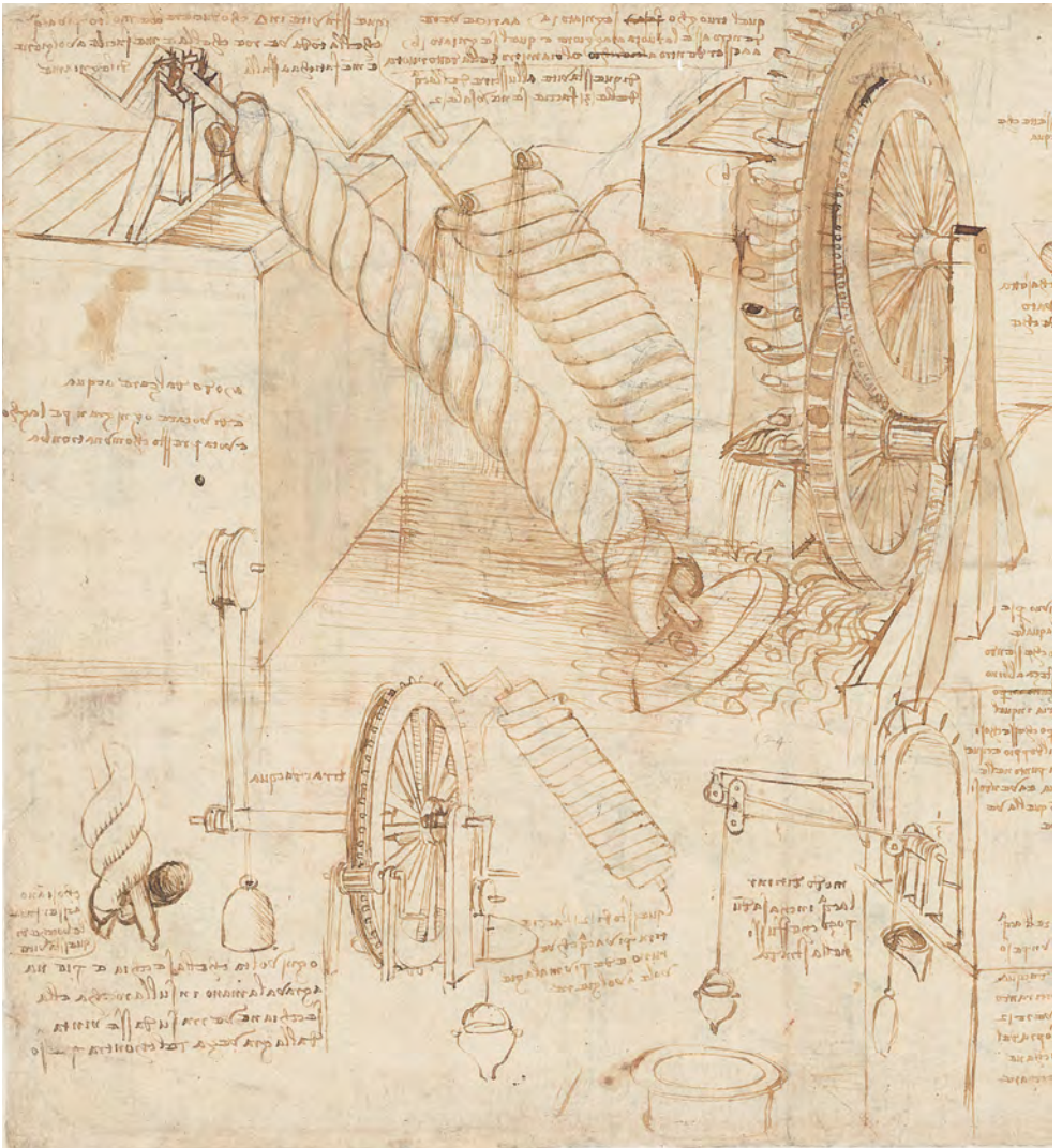
Fig. 55. A perpetual-motion machine using a water screw.
