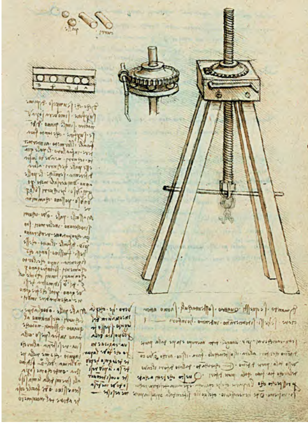
Fig. 56. A screw jack with ball bearings.
